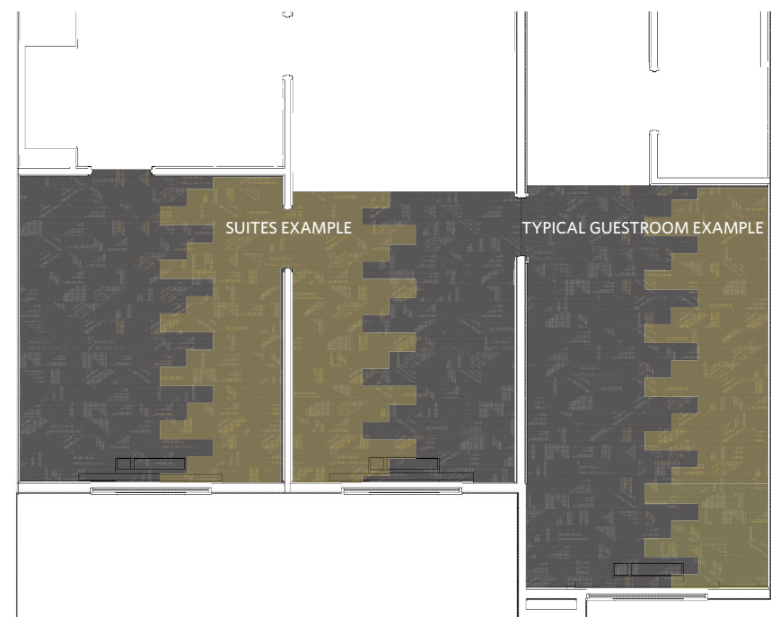
Guest Room Field and Accent, 25cm x 1m. 1/3 Staggered Installation.
