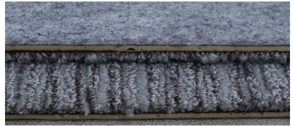
Close up of carpet tiles, showing face, edge and backing.
