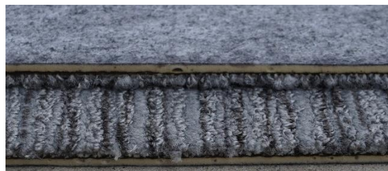
Close up of carpet tiles, showing face, edge and backing.
