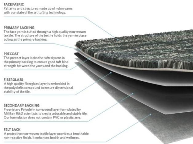
Figure 1. Illustration of Milliken Carpet Tile Construction
