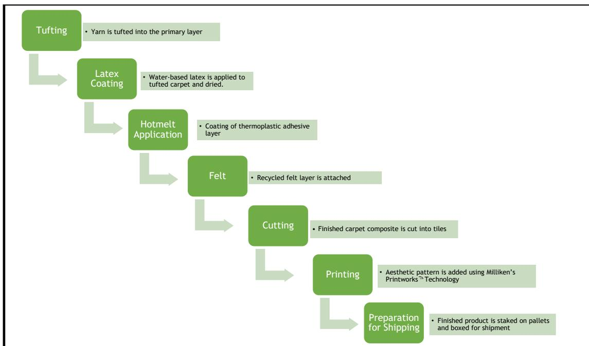
Figure 2. Production process for Milliken Carpet Tile
