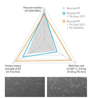
Scanning electron microscopy images show more finely dispersed and uniform size of ethylene-based polymeric islands in the recycled PP matrix when modified with Exact POE and DeltaMax performance modifiers (right) compared to unmodified recycled PP (left).
