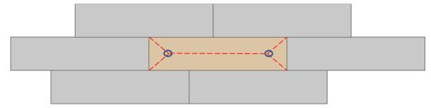
d. Using a small flat screwdriver or chisel, insert the head into intersection, indicated by the blue circle in the figure, and gently pry the corner of the first small triangle piece up. Insert a larger flat screwdriver or chisel to lift the triangle piece. Gently work the piece away from the joint. USE SPECIAL CARE TO PREVENT DAMAGE TO THE EDGES OF THE SURROUNDING TILES.
