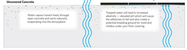
**Water can cause all kinds of problems.** Moisture seeks equilibrium. It essentially just wants to evaporate. Water vapour will naturally rise until something gets in its way. Concrete is filled with vertical capillaries and does not hinder the process.
