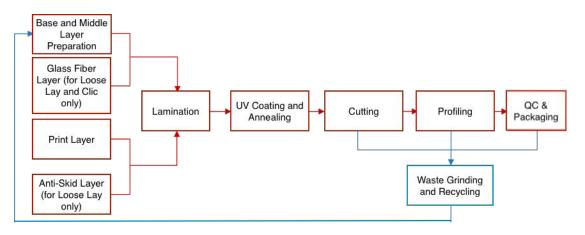
Figure 2. Production Process of the Milliken Fortified Foundations 2.5 mm and Fortified Foundations 5.0 mm
