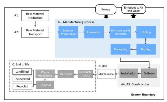
Figure 3. System Boundary of LCA study
