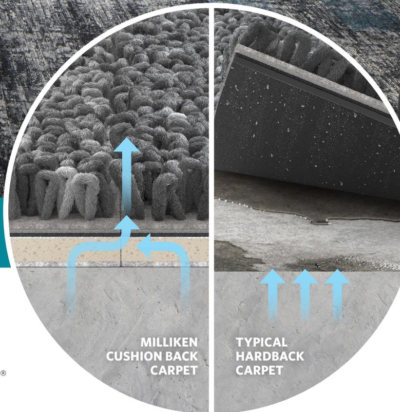
*With Milliken carpet, moisture vapour can travel freely through our open-cell cushion backing, venting naturally from the seams. Hardback carpet often traps moisture vapour, causing water condensation to form underneath the tiles.*
