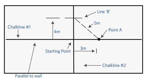
gives a line exactly 90° to chalkline #1. This line should be extended to entire length of the area as indicated.
