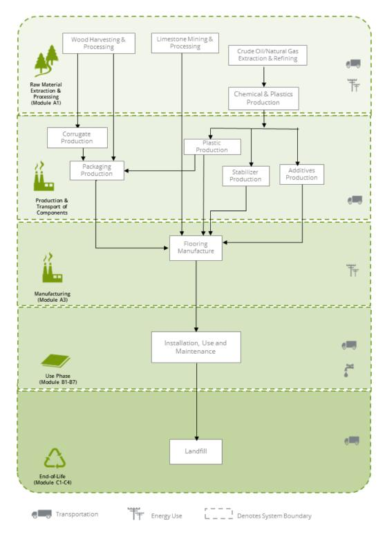
**Figure 1.** Flow diagram for the life cycle of the Merge Forward Polypropylene Composite Tile flooring products.
