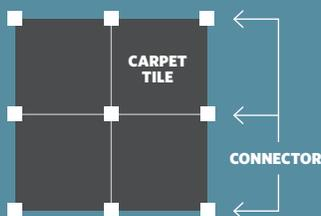
TractionBack® Plus connectors are centered under each corner of the tile, regardless of tile size or installation method.
