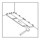
end (right side). Align joint on left side, slide plank to left by hitting tapping block placed in right end.
