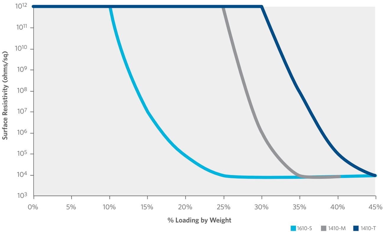
This example illustrates the ability to control the desired surface resistivity in epoxy resin by Zelec® ECP selection and loading.
