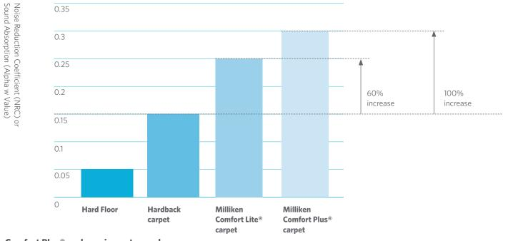
Comfort Plus  $^{\mbox{\tiny (e)}}$  reduces impact sound (e.g. from foot traffic) by up to 40%
