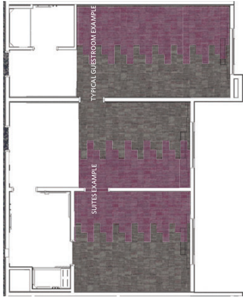
Guest Room Field and Accent, 25cm x 1m, 1/3 Staggered Installation.
