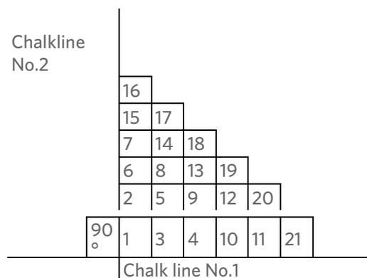
**Monolithic** - Arrows on the back indicate pile direction. These should all be in the same direction.
