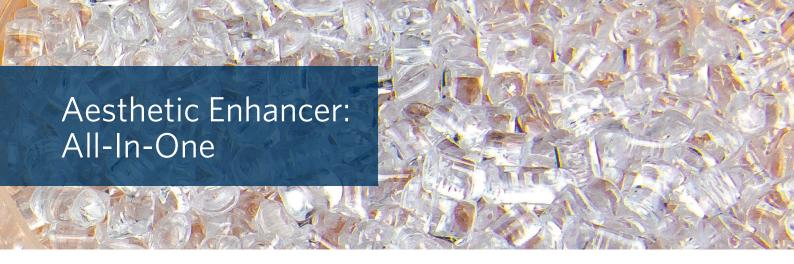
Amorphous transparent polymers often have a yellow appearance due to the production technology used to make them. These polymers tend to be color tuned with very low loadings of optical brighteners and/or solvent dyes. KeyPlast's aesthetic enhancer can help here, with its innovative anti-yellowing package. Offering purity, consistency and traceability, these additives – combined with Milliken's strong regulatory and technical support – can help a brand to protect its all-important image.
